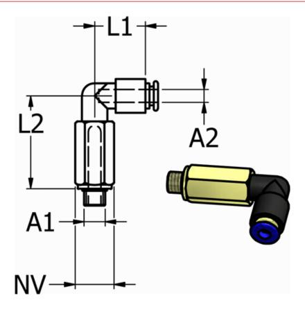
Ext. hose diameter A2 = 6 mm L1 = 32 L2 = 18.6 NV = 10 Thread A1 = M6
